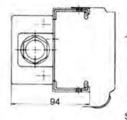
This part is fitted into a 1 Mtr track section with a sheet steel cover, cable connectors for cable sizes 25 to 120 mm². The isolating blocks are made of glass fibre material with connecting studs for power feed at each side for conductors nos L1, L2, L3. Copper joint sleaves are used for PEN with connecting studs. Type no. TRM 4/2/140 A
