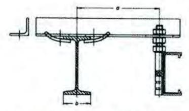
a) Fitting from the girder with moveable girder clamp measurment A may be determined by yourself.
