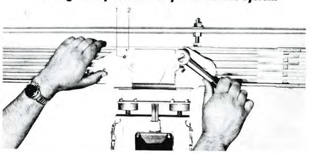
Trolley collector can be inserted into the system anywhere (Warning isolate power).
