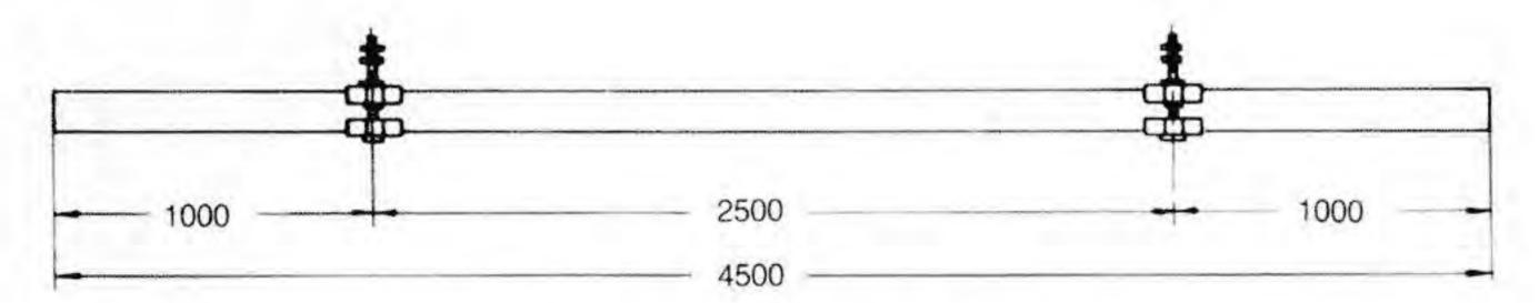
3 supporting brackets are to be used on a standard leg of 4500 mm length, if there is an additional mechanical load of up to 50 kilograms per meter of bus way.
