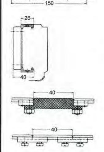
With isolating blocks made of glass fibre material for conductors nos. L1, L2, L3 and N.
