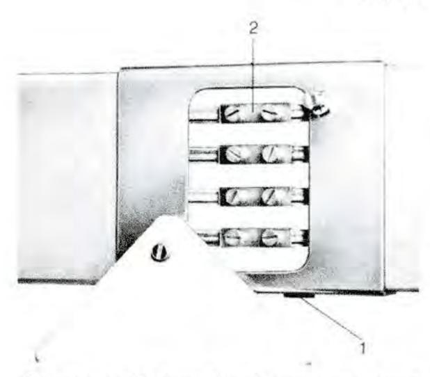
Fasten joint plate to lower side of C-frame with flat head screws (1).
