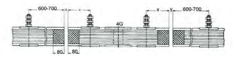
X = Suspension hangers distance must be between 600 - 700 mm
