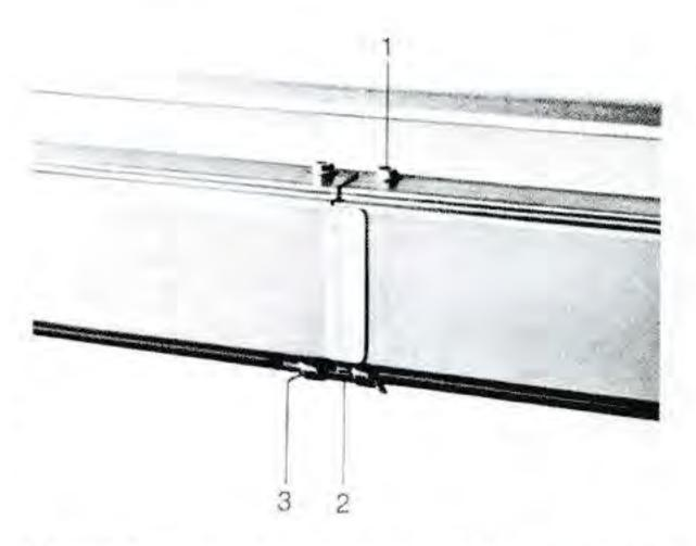
Cover is fastened with pawl screws (1) to C-frame's top side. Two lengths of cover are coupled together at the joint with the help of a latch bolt (2). To secure its pin, center part of it is bent outward slightly.
