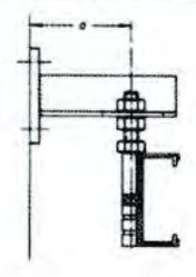
Wall and side fixing bracket
