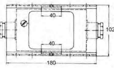
Sheet metal housing and cover galvanized. This section may be installed between any two lengths. Total length of system will increase by 40 mm. This isolating blocks are of glass fibre material and connecting studs for power feeds at each side for conductors
