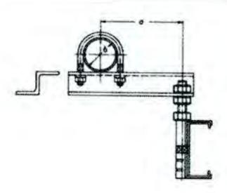
D) Fitting from a tube with moveable U clamp measurement A may be determined by yourself. Please state in your order the diameter of the tube and that of the suspension bolt.
