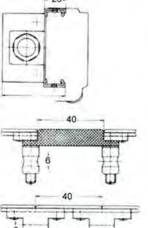
With isolating blocks made of glass fibre and connecting studs for power feed at each side for conductors nos. L1, L2, L3 and N.
