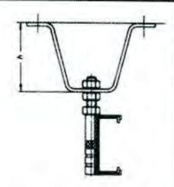
c) Roof fixing with V bracket
